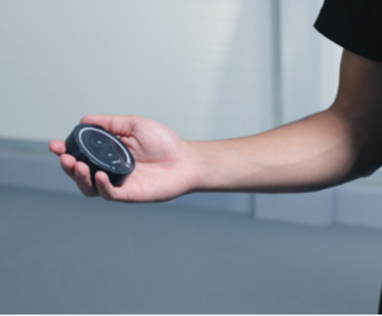
Remote control for lighting (on/off and dimming functions)
