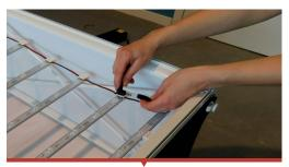
3. Connect the adapter to the lighting plug on the bottom side.
