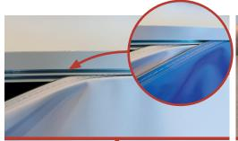
**2.** For the sides, use the inner groove for the block-out. The outer groove is for the print.
