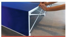
**10.** Work your way around the frame until all silicone edges are attached.
