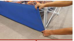
9. Start in the 4 corners of the frame, to divide the tension.
