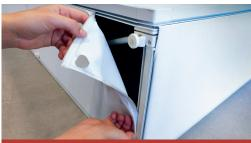
**3.** The block-out with holes goes over the adjustable feet at the bottom of the frame.
